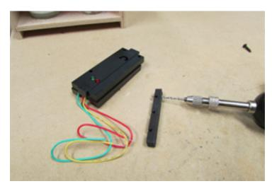
Figure 1 – You are going to need attach the DZ-1000 switch motor to an extra tie bar. Any scrap piece of wood or plastic tie bar will do. In this case the tie bar came from a discarded Gargraves track. First locate and drill a pilot hole for the size screw you will be using. Use screws that are long enough (Atlas O track screws or any 3/4 inch #3 or 4 screw will do) so that when placed into position the motor can be secured to the train board.
