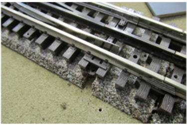
Figures 2 and 3 – Disconnect the switch motor wires then remove any screws holding the Atlas O switch motor down. There are two tiny bolts that hold the switch motor to the track which must be removed. Note there are tiny nuts on the bottom of the track ties. Try to retrieve these as they could move around later and may cause a track short.
